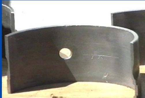
Piston-rod bearing from our 30,000 hours old engine with **Polytron MTC** totally clean with almost no wear at all.
