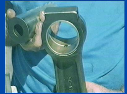
After 30,000 hours in operation and 100 hours in the presence of water, all piston pin bearings didn't have any wear and looked like new.
