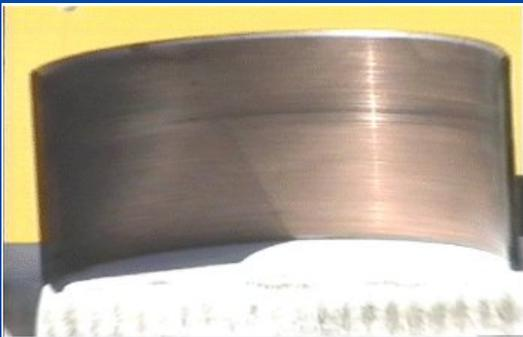
Piston-rod bearing from 16,000 hours old engine, (without **Polytron MTC**) chewed up as a result of wear.
