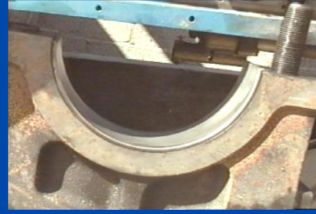
Crankshaft Main Bearings looked like new, there were no traces of wear. They maintained their original coating. Usually after 17,000 hours they are chewed up. In this engine we used **Polytron**, so there was almost no wear at all after 30,000 work-hours.
