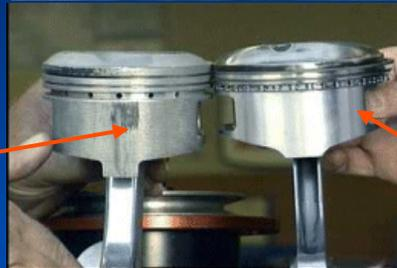
The piston on the right was taken out from an engine after 350 runs with Polytron MTC. The piston has no signs of wear, is totally clean, and all the friction surfaces are polished.
