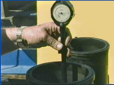
There was almost no wear on the liners and the dimensions were within the manufacturer's specs.
