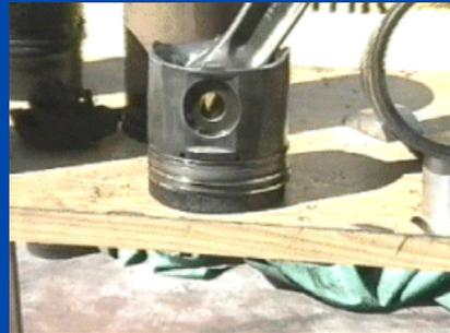
All the pistons had piston skirts and piston rings totally clean of any build-up. The rings looked like new and didn't have any wear.
